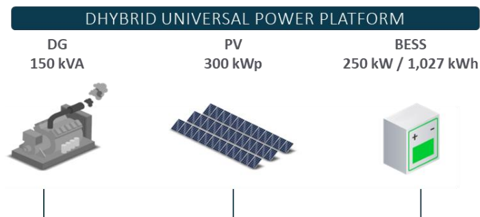
Figure 1: Cheetah Plains System Configuration
